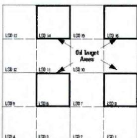
Together, the oil and gas target areas overlap and form a **common target area**, as shown in the shaded portions of the figure below. Many companies prefer to drill the common target area if there is a chance to encounter both oil and gas.
